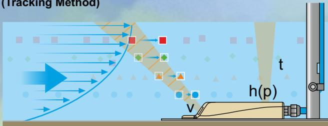
Scatterers (particles, minerals or gas inclusions) present in the medium are scanned with ultrasonic impulses and stored as an echo pattern. Further scans take place in the millisecond range. The position of the particles is determined via the transit time of the ultrasound. A comparison of the time-delayed signals allows the flow velocity to be calculated. This results in a profile of the flow velocities from the bottom to the surface.
