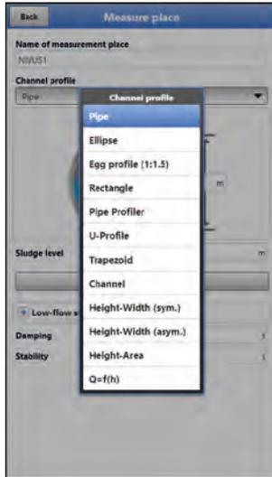
**Fig. 36-2 Selectable channel profiles**
