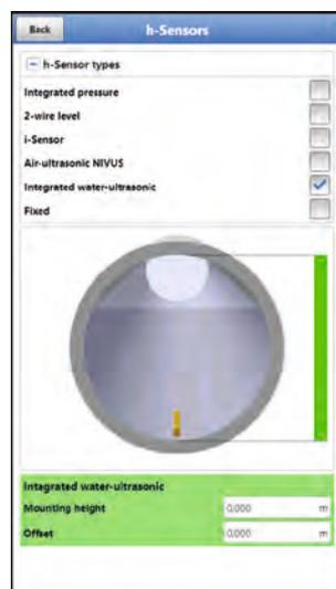
**Fig. 36-7 Selection level sensor settings**
