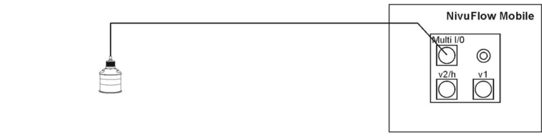
Fig. 25-3 Connection of level sensor i-Series and NivuBar Plus
