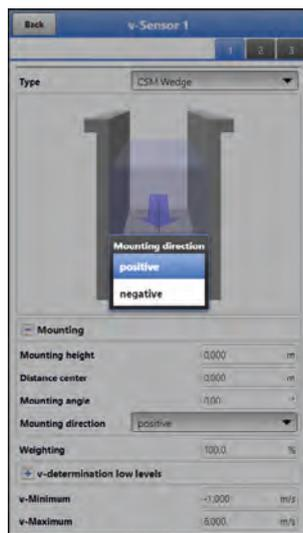
**Fig. 36-19** Modifying the sensor mounting direction
