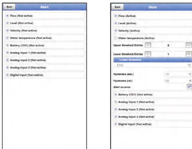
**Fig. 43-4 Water temperature**
