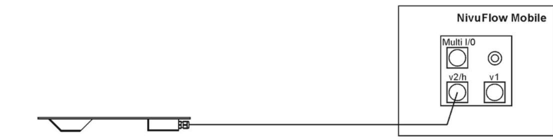
Fig. 25-2 Connection of level sensor DSM-L0
