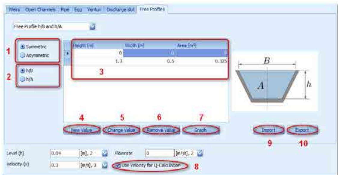
Figure 124: Configuration dialog for a free profile
