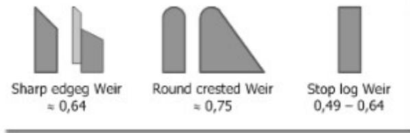
Figure 111: Examples for typical Overfall Coefficients
