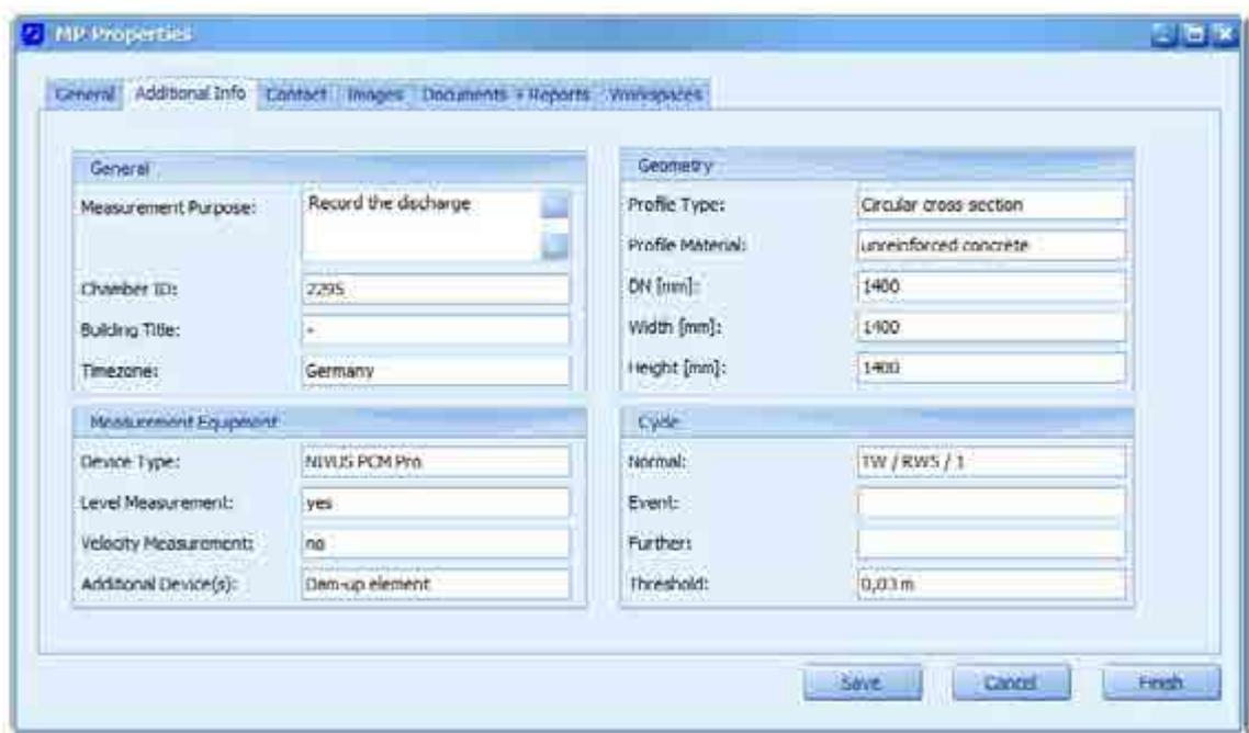
Figure 46: Additional Information of a measurement place
