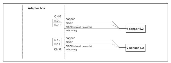
Fig. 5-11 Connecting flow velocity sensors (Path 6)
