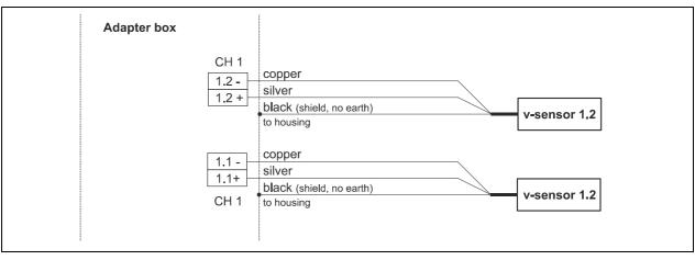
Fig. 5-6 Connecting flow velocity sensors (Path 1)
