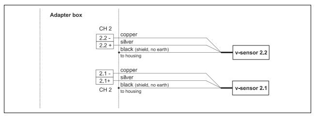
Fig. 5-7 Connecting flow velocity sensors (Path 2)
