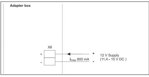
Fig. 5-17 12 V DC model power supply
