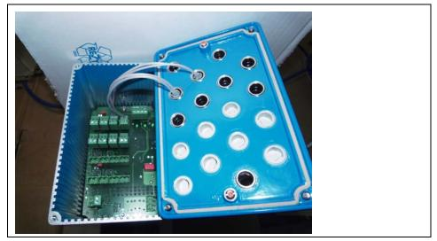
Fig. 5-25 General view sealing cover with connection board
