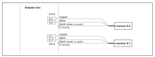
Fig. 5-13 Connecting flow velocity sensors (Path 8)
