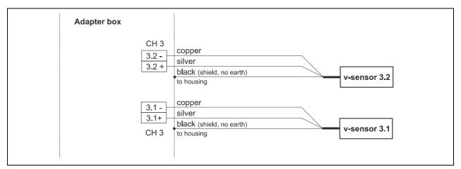
Fig. 5-8 Connecting flow velocity sensors (Path 3)
