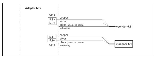
Fig. 5-10 Connecting flow velocity sensors (Path 5)
