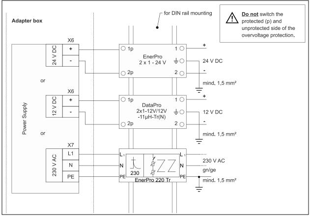
Fig. 5-18 Connecting the overvoltage protection
