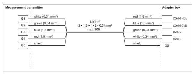
Fig. 5-14 Connection adapter box to measurement transmitter
