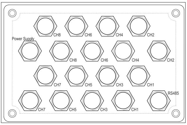
Fig. 5-2 Overview cable glands / measurement paths
