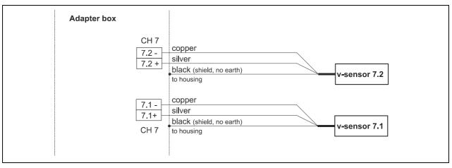
Fig. 5-12 Connecting flow velocity sensors (Path 7)
