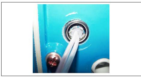
Fig. 5-23 Inserted sensor cable - inside view
