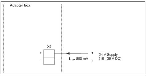
Fig. 5-16 24 V DC model power supply
