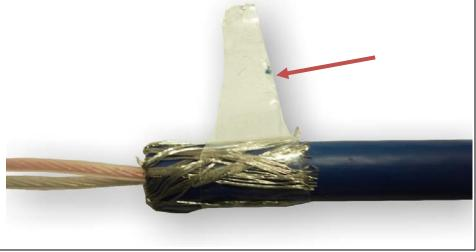
Fig. 5-20 Peel off the transparent tape
