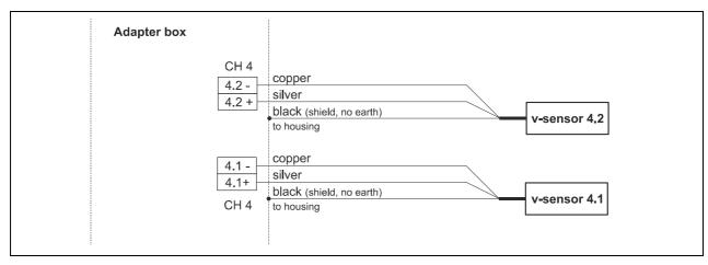
Fig. 5-9 Connecting flow velocity sensors (Path 4)
