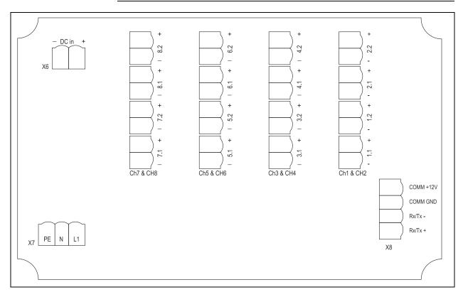
Fig. 5-5Adapter box wiring from serial number 1148NIZ0076 onwards
