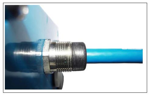
Fig. 5-22 Inserted sensor cable – detailed outside view
