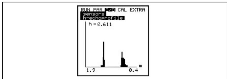
**Fig. 8-106** Screen level measurement echo profile
