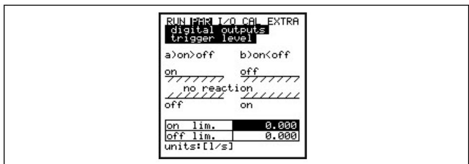
**Fig. 8-69 Relay trigger level settings**
