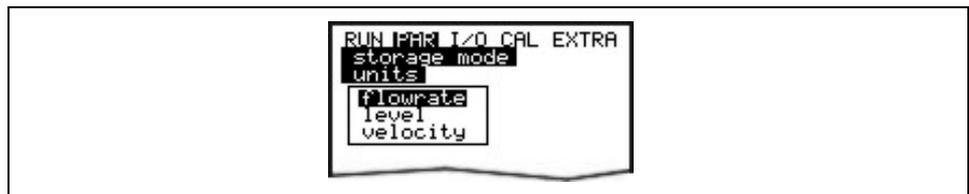
Fig. 8-82 Selecting the measurement value in storage mode
