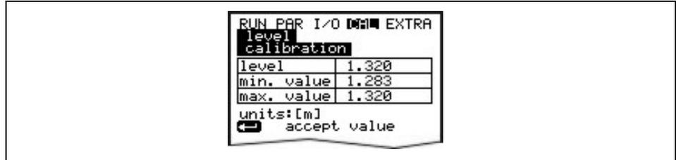
Fig. 8-119 Level screen - calibration
