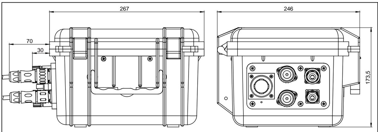
Fig. 6-1 PCM 4 enclosure dimensions and connection sockets
