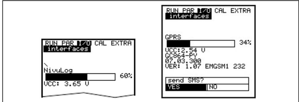
Fig. 8-108 Signal quality screen NivuLog PCM and GSM-Module
