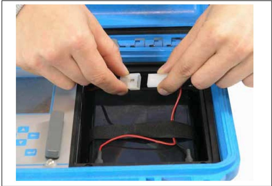
**Fig. 6-8 Plug connection to rechargeable battery**
