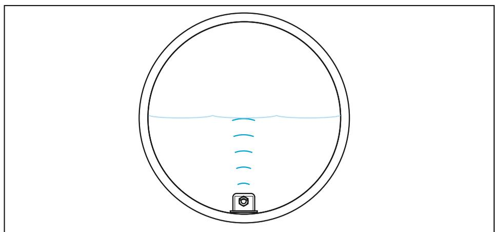
**Fig. 8-46 Sensor type 2: Water-Ultrasonic NIVUS**
