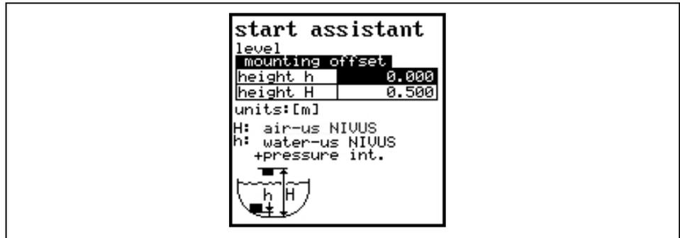
Fig. 8-11 Modifying the mounting offset of level/height sensors
