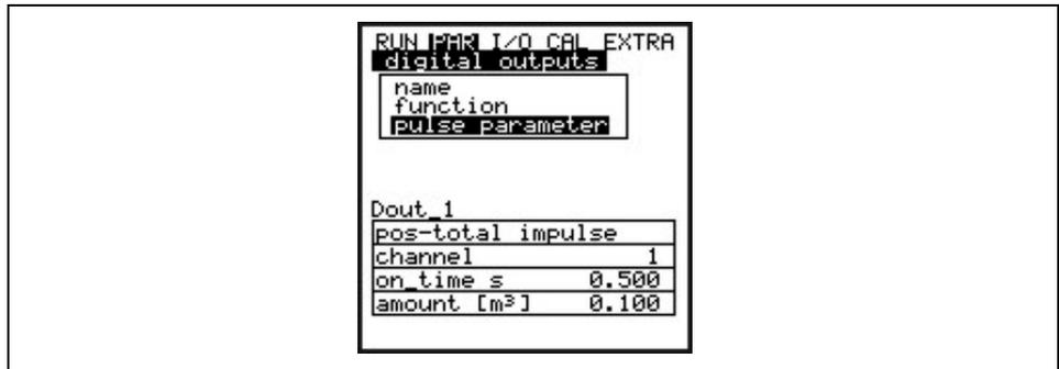
**Fig. 8-70** Setting relay impulse parameters
