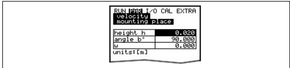
>height h< mounting height of the sensor body.
