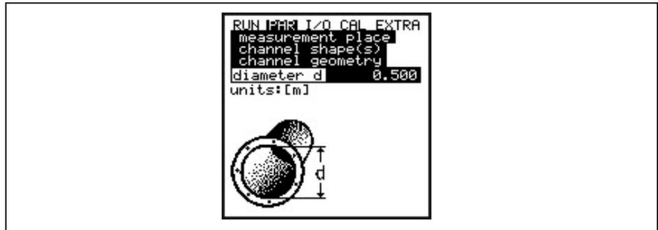
Fig. 8-34 Setting the channel geometry in pipe profiles
