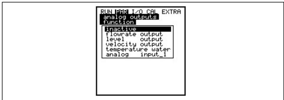
**Fig. 8-64** Selecting analog output functions
