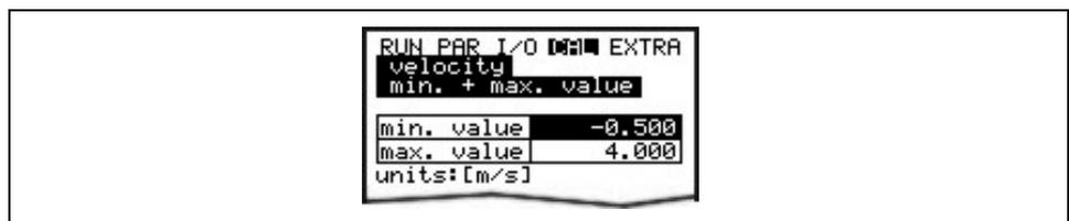
Fig. 8-124 Measurement range of flow velocity
