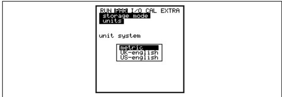
Fig. 8-81 selecting the unit system in storage mode
