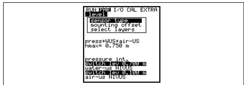
Fig. 8-43 Level measurement – submenu
