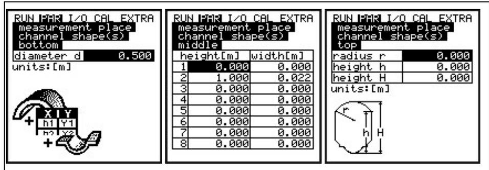
Fig. 8-39 Profile Dividing into three zones
