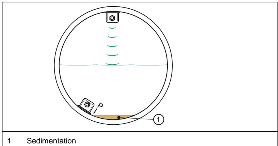
**Fig. 8-49 Combination: Air-Ultrasonic and pressure int.**
