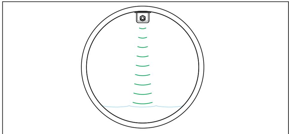
**Fig. 8-45 Sensor type 1: Air-Ultrasonic**
