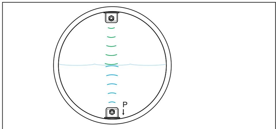
**Fig. 8-52 Sensor type Air-US, Water-US and Pressure**
