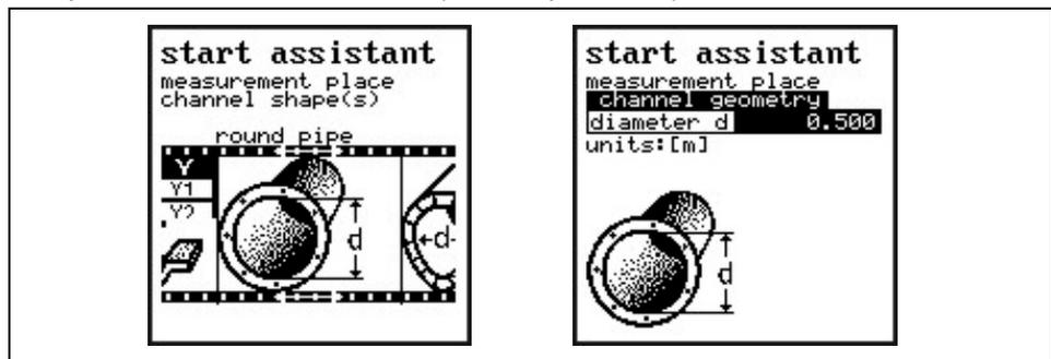
**Fig. 8-8 Channel shape and channel geometry selection**
