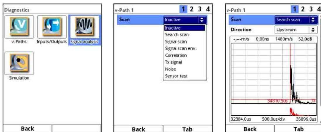
Fig. 41-1 Signal analysis Pulldown menu / search scan
