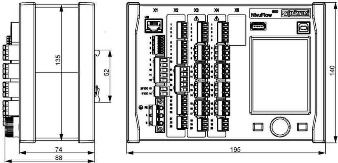
Fig. 15-2 Dimensions of NivuFlow 600 enclosure type E0
