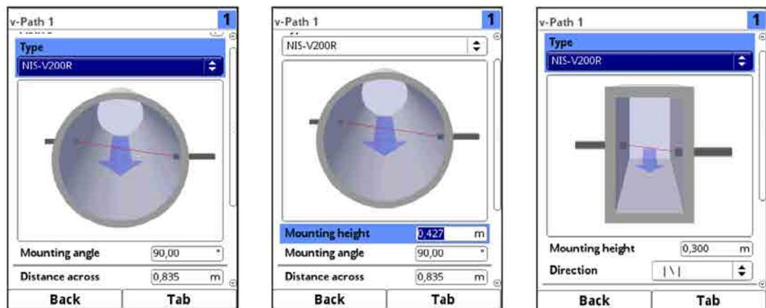
**Fig. 31-11 Sensor mounting “Insertion” in pipe or rectangle**
