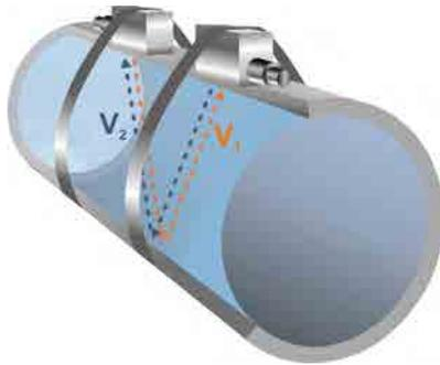
**Fig. 31-3 1-Path measurement, path arrangement: "Diametral V"**
