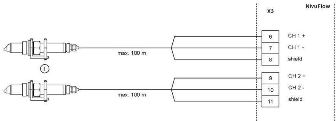
1 Connectable flow velocity sensors
