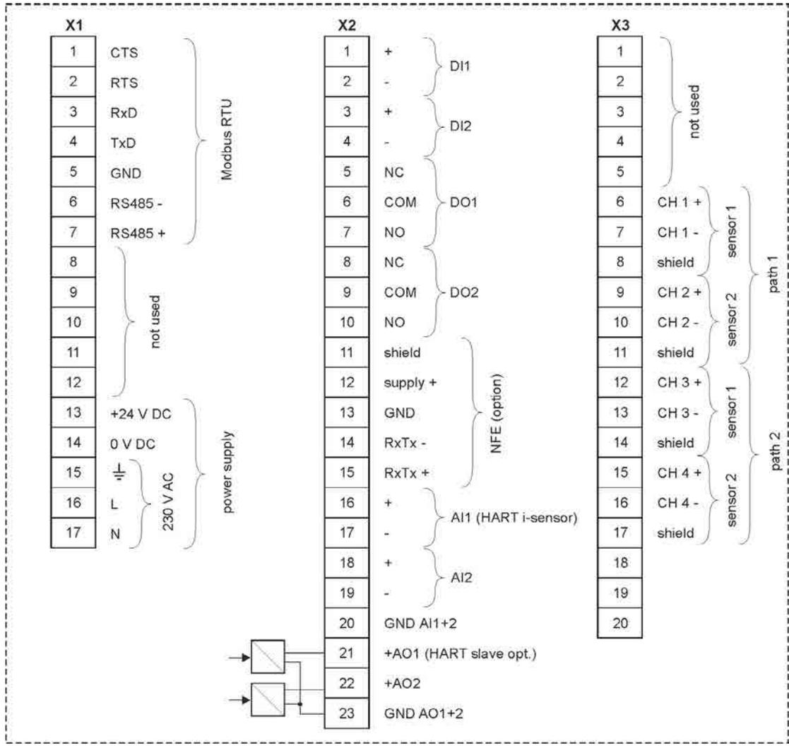
**Fig. 21-2 Terminal connections NivuFlow 600 Type T2**
