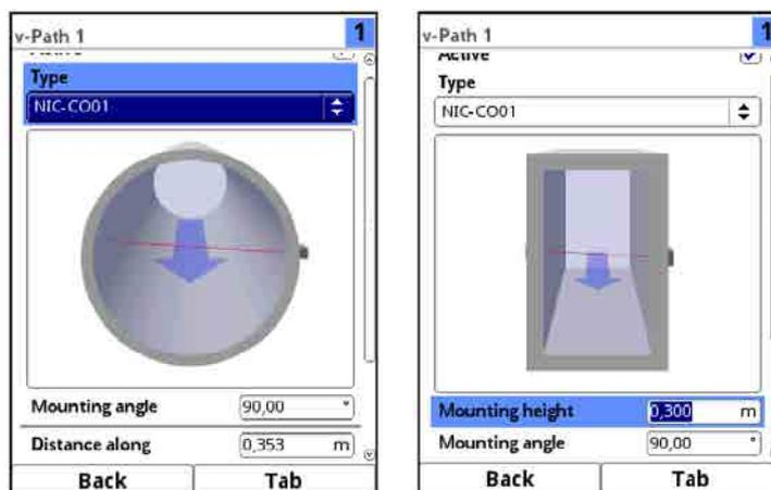
**Fig. 31-10 “Clamp-On” sensor mounting in pipe or rectangle**
