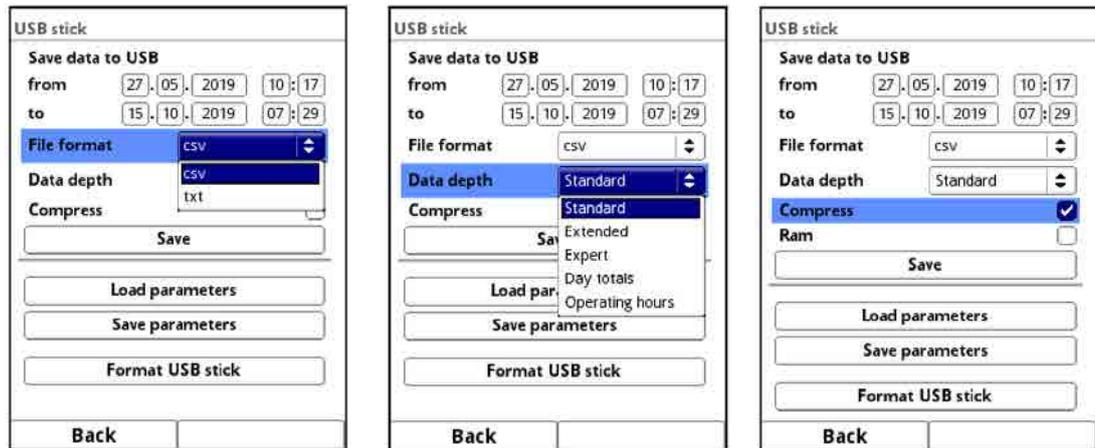
**Fig. 32-7 Transmission period / data depth / compression**
