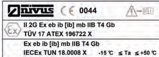
Fig. 17-2 Nameplate NivuFlow Mobile 600 Ex-Version (additionally)
