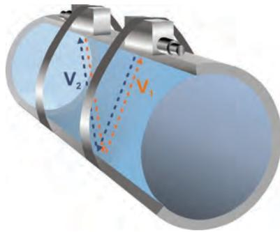
**Fig. 38-2 1-Path measurement, path arrangement: "Diametrical V"**
