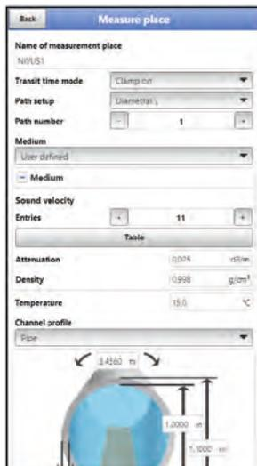
**Fig. 38-3** Selecting the measurement medium
