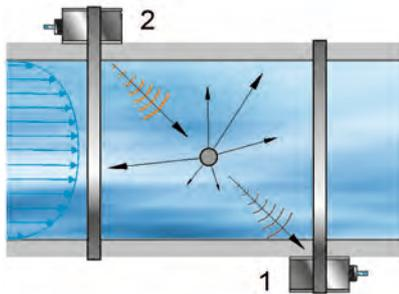
Fig. 20-1 Signal damping due to interfering particles
