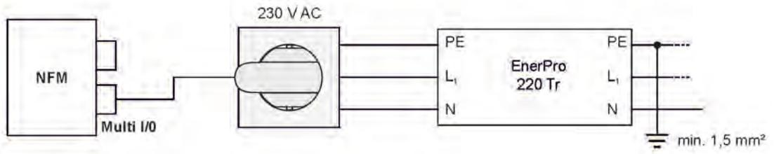
Fig. 25-3 General overvoltage protection for AC power supply
