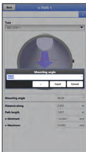
**Fig. 33-4 Enter the mounting angle (Clamp-On)**
