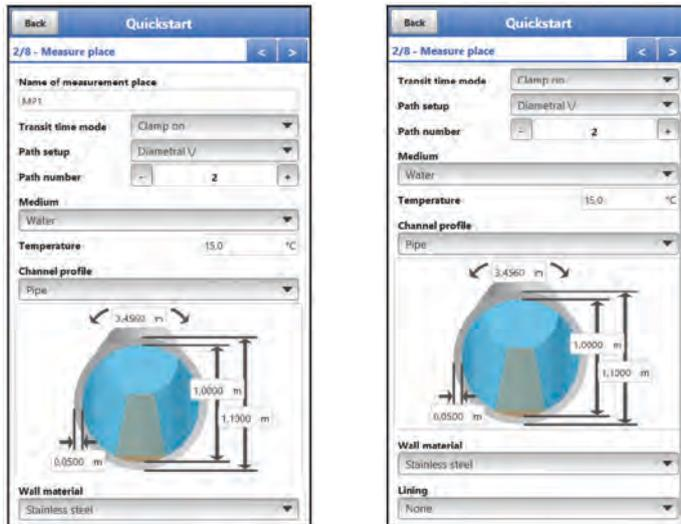
**Fig. 44-2 Measurement Place**
