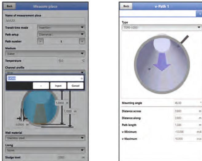
**Fig. 24-5 Entering pipe dimensions and mounting angle**
