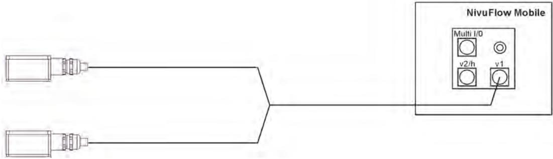
Fig. 25-1 Connection of flow velocity sensors, 1 pair/path
