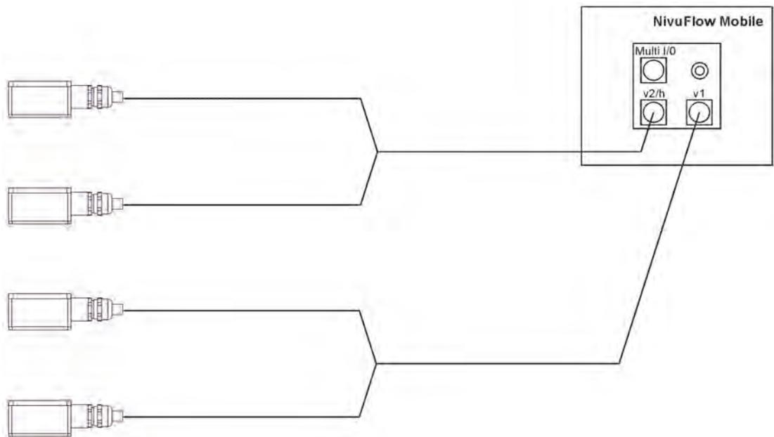
Fig. 25-2 Connection of flow velocity sensors, 2 pairs/paths
