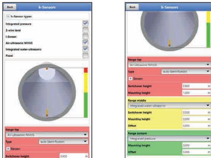
Fig. 36-8 Level sensor selection
