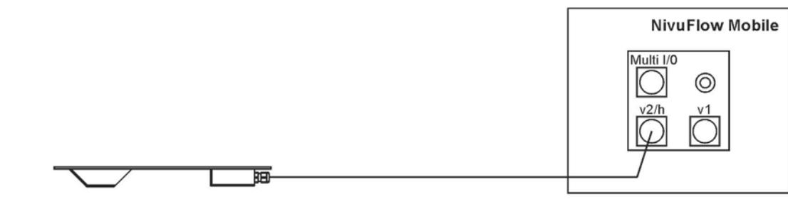
Fig. 25-2 Connection of level sensor DSM-L0
