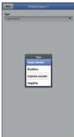
**Fig. 36-26 Digital input activation**
