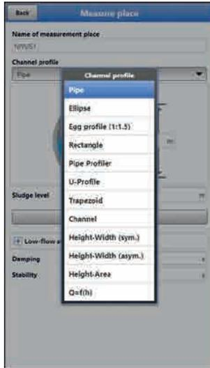
**Fig. 36-2 Selectable channel profiles**
