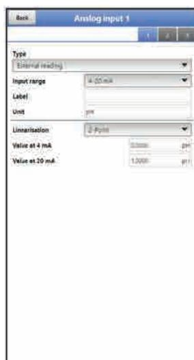
**Fig. 36-24 Analog input as external reading**
