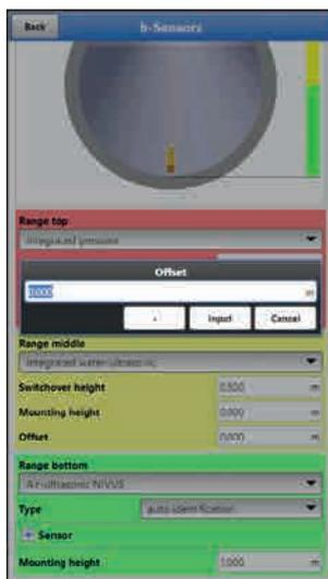
**Fig. 36-12 Programming integrated pressure sensor**
