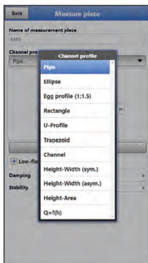
**Fig. 38-2** Selectable channel profiles
