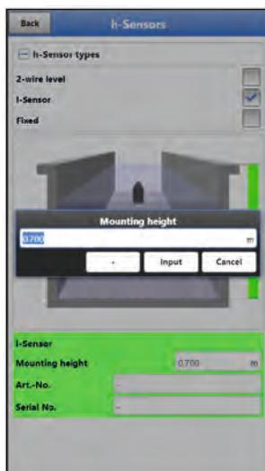
**Fig. 33-2** Selecting the h-Sensors / specifying the mounting height
