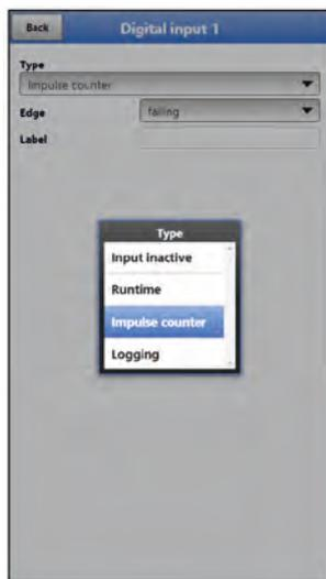
**Fig. 38-13 Digital input activation**
