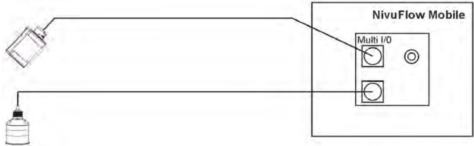
Fig. 25-1 Connection of Radar sensor and i-Series sensor
