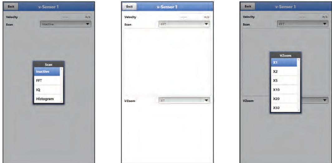
**Fig. 50-1 Signal analysis selection menu / FFT / IQ**
