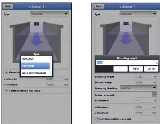
**Fig. 33-3** Selecting the v-Sensors / specifying the mounting position
