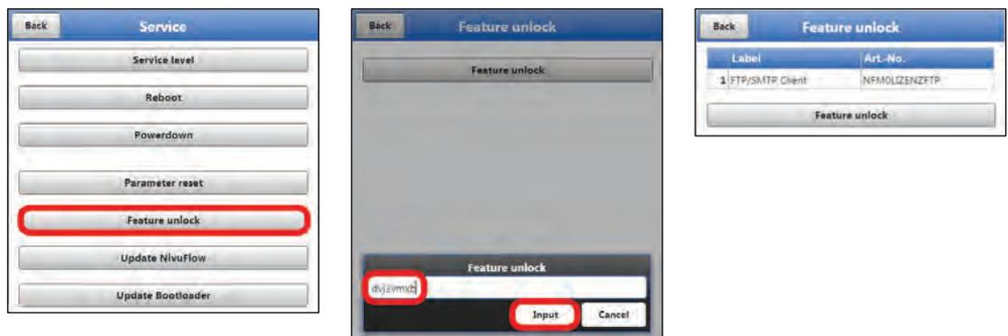
**Fig. 40-10 Licence activation in NFM display tool**
