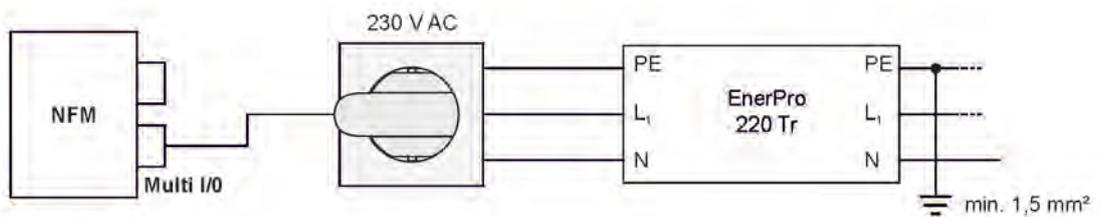
Fig. 25-2 General overvoltage protection for AC power supply
