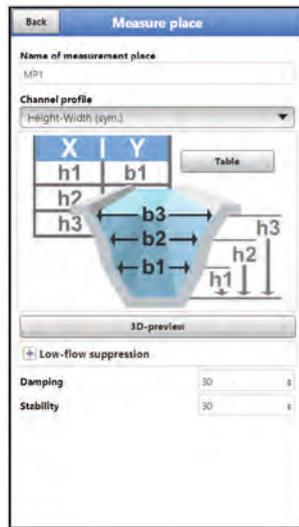
**Fig. 38-4** Setting of profile using height-width (sym.)
